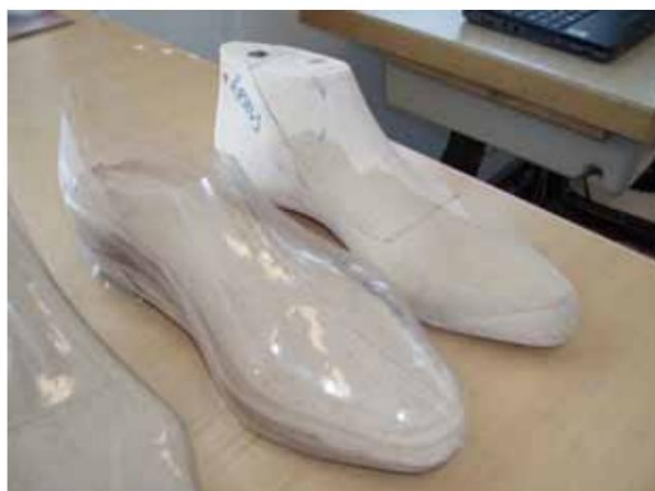
Fig. 14. Orthopedic school reading. Today, the orthopedist measures and describes the customer's foot or takes an impression over which the last is made. This is returned to the orthopedist covered with a hard plastic shell. With this transparent "shoe" around the customer's foot, the last corrections are described and the last is sent for correction.
